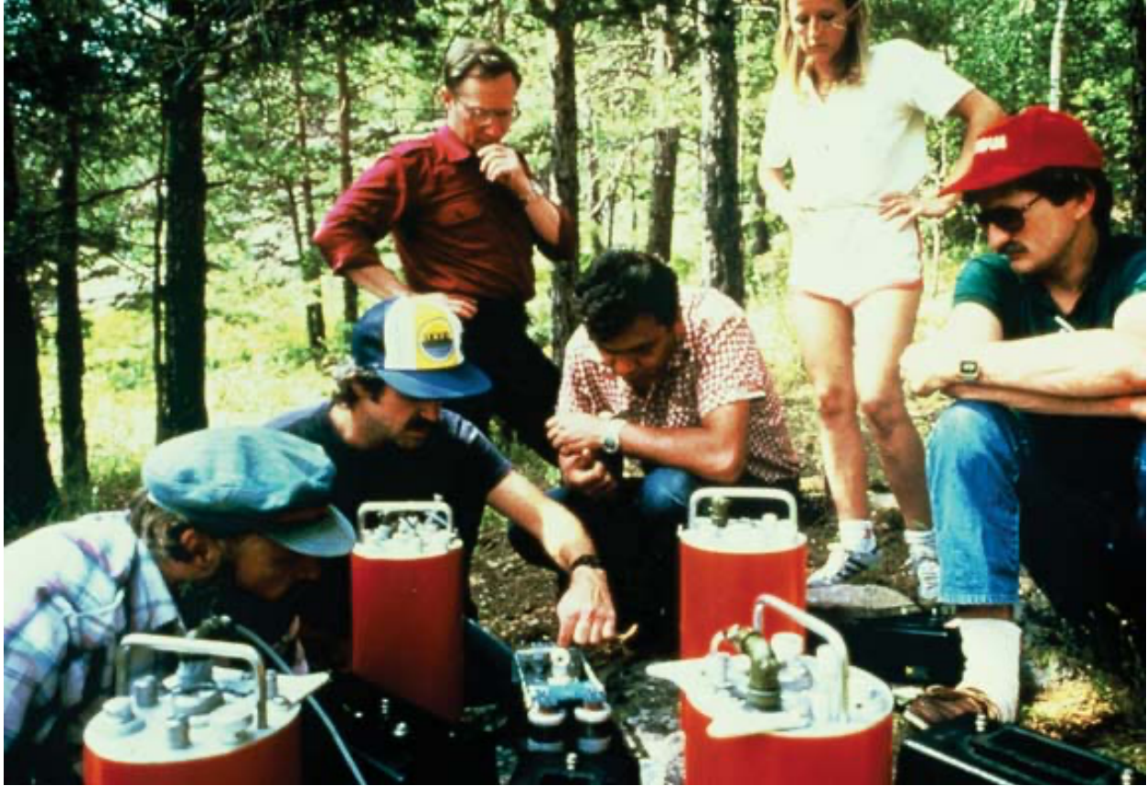
A team of seismologists sponsored by the Natural Resources Defense Council setting up portable surface seismometers near the Soviet Semipalatinsk test site in Kazakhstan, July 1986. (NRDC)
